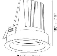
Ø 144mm 5 <sup>1</sup>/<sub>16</sub>" Ø 182mm 7 <sup>3</sup>/<sub>16</sub>"
